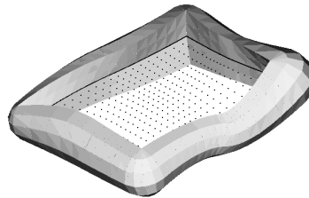
Figure 30: A medial patch inside its associated solid
